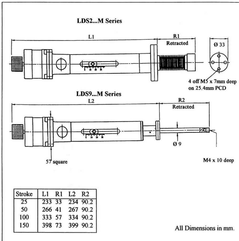
**Figure 11- LDS2...M and LDS9...M Motor Driven Linear Motion Drives**
