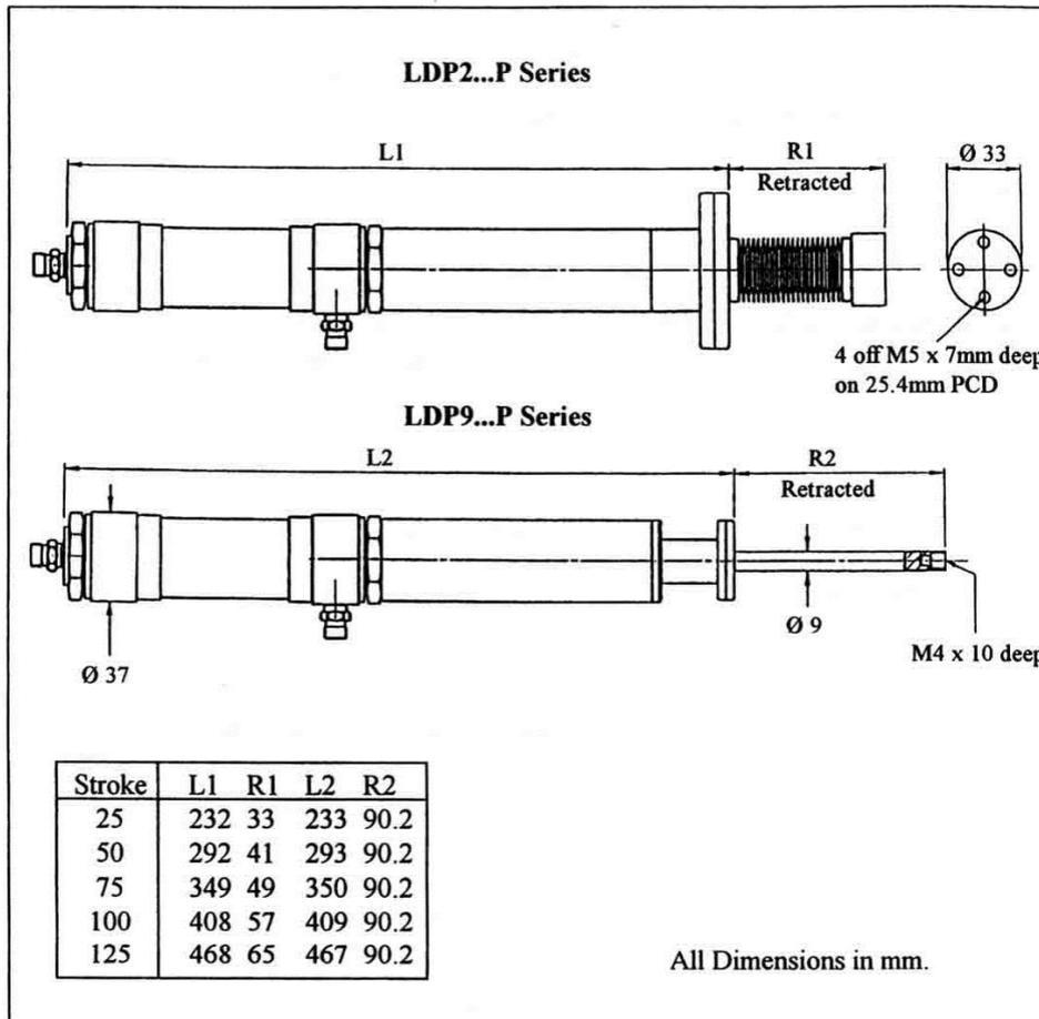
Figure 8 - LDP2...P and LDP9...P Pneumatic Linear Motor Drive
