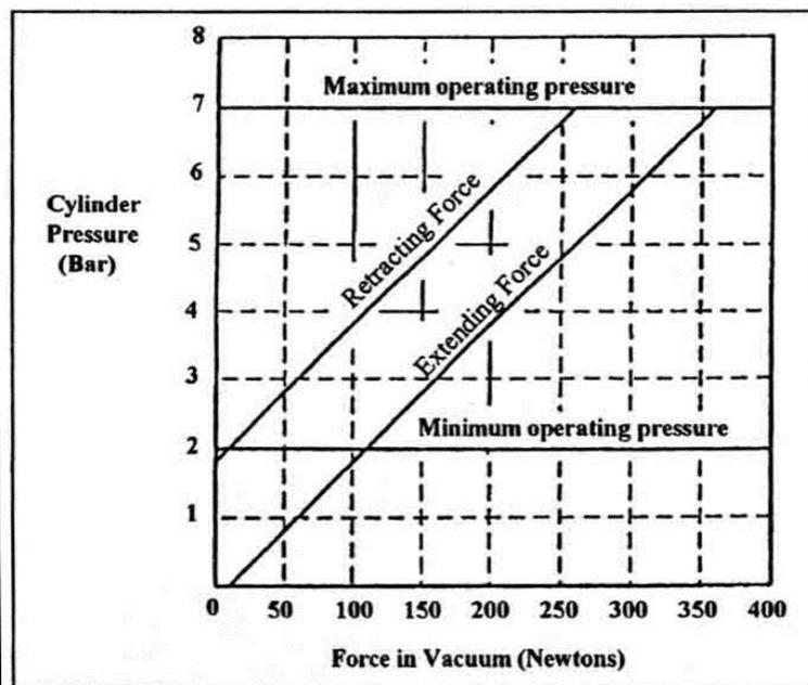
Figure 10 - Pull/push Forces vs. Cylinder Pressure
