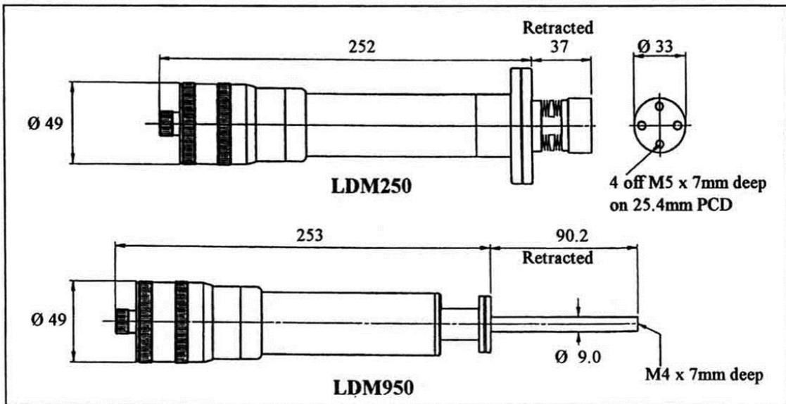
Figure 6 - LDM250 and LDM950 Micrometer Linear Motion Drives
