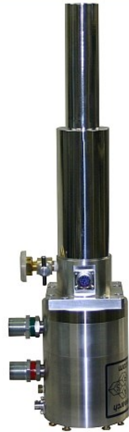
The above picture shows a cryocooler with a vacuum shroud, radiation shield, and sample holder installed.
