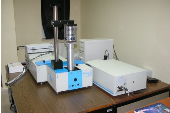
CS202SE-DMX1-AL Installed on Jobyn Yvon Spectrometer.
