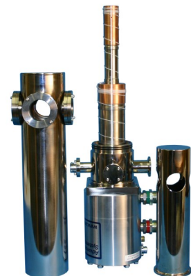
The above picture shows a coldhead, vacuum shroud, and radiation shield.
